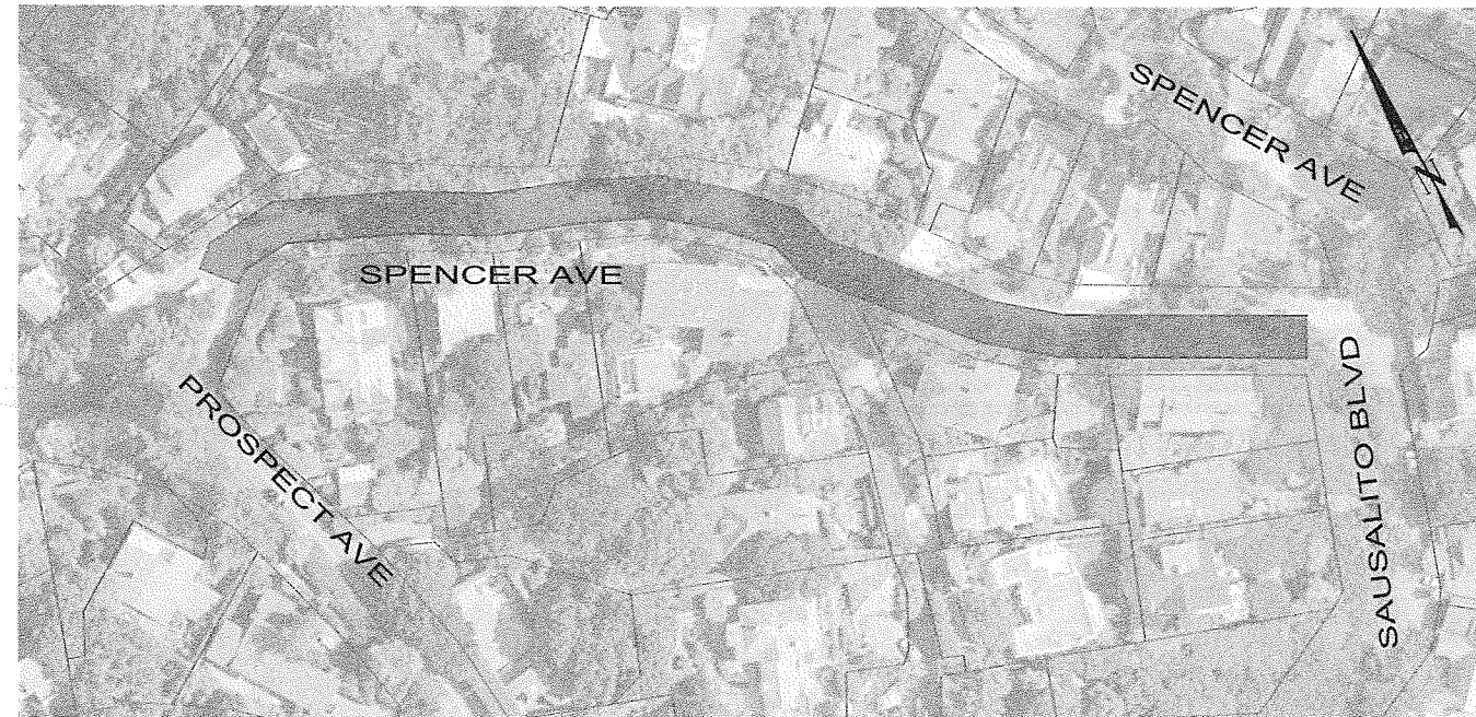
SECTION 6: SPENCER AVE (PROSPECT AVE TO SAUSALITO BLVD) TREATMENT: CRACK SEAL & CAPE SEAL
