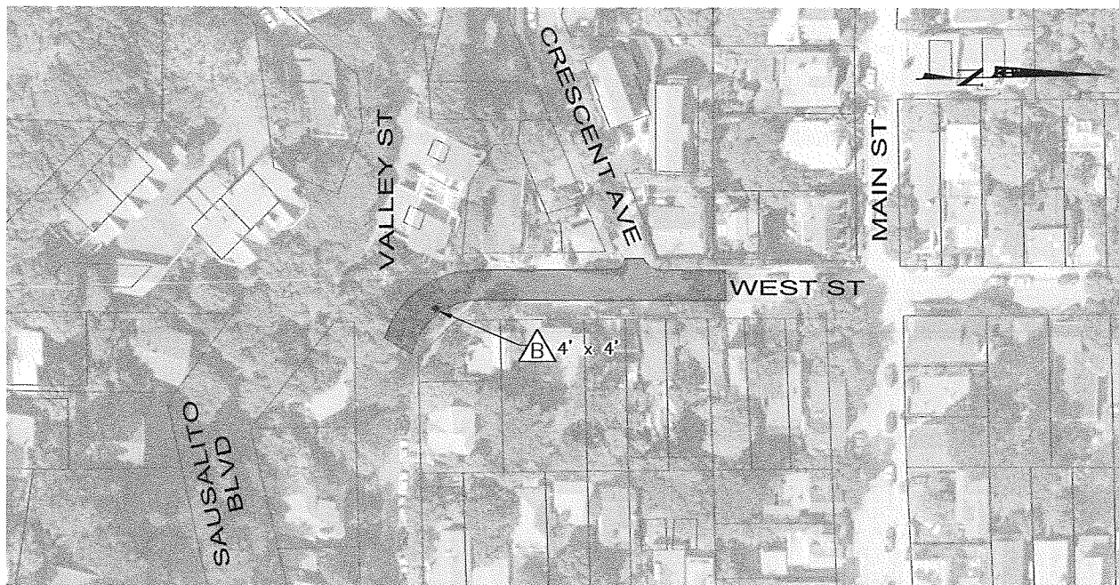
SECTION 11: WEST ST (VALLEY ST TO BRIDGE) TREATMENT: CRACK SEAL & CAPE SEAL
