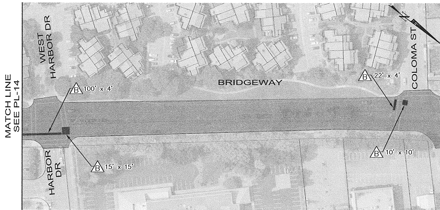
SECTION 18: BRIDGEWAY (PRINCESS ST TO NORTH BRIDGE BLVD) TREATMENT: CRACK SEAL
