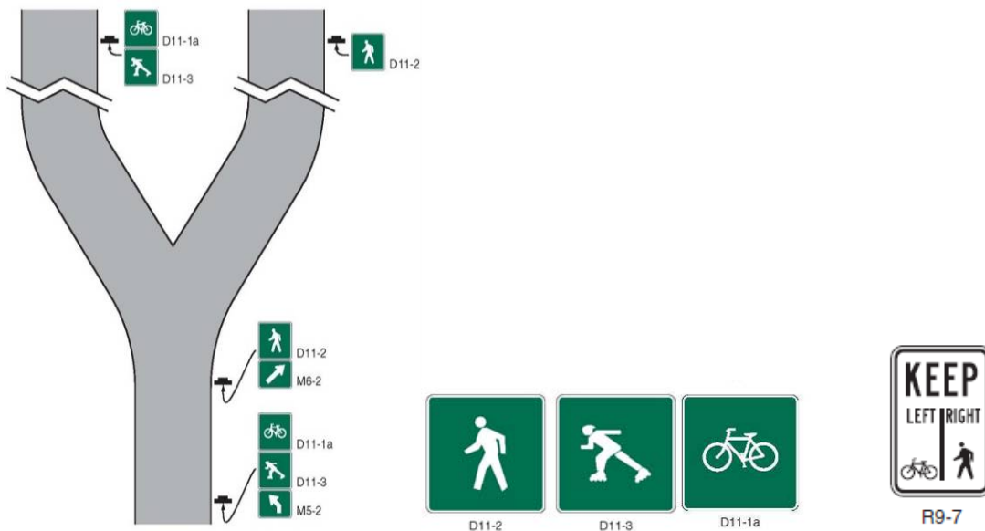
Figure 6-3 2009 MUTCD Example of Mode-Specific Guide Signing on a Shared-Use Path (left) Shared-Use Path Guide and User Permitted Signs (middle) and Shared-Use Type Restriction Sign (right)
