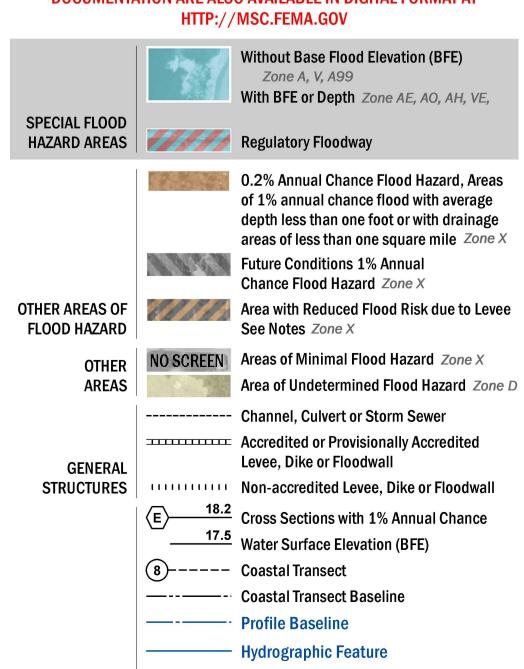
→ 513 → Base Flood Elevation Line (BFE)
