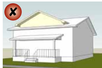
Full Gable Dormer Gable overwhelms the facade and alters the character.
