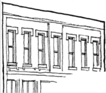
Existing building with missing cornice.
