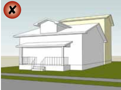
Two-and-a-half story addition with connector Addition is set back behind the original and accessed by a connector.
