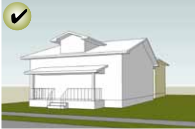
One-and-a-half story addition with connector Addition is set back behind the original and accessed by a connector.
