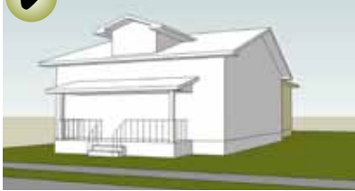
One story attached addition Addition is set back behind the original building.
