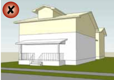
Two-story roof-top addition Addition is set back behind the original and accessed by a connector.
