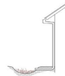
Downspout to vegetated area. The head from the roof height makes it possible to route roof drainage some distance away from the building.
