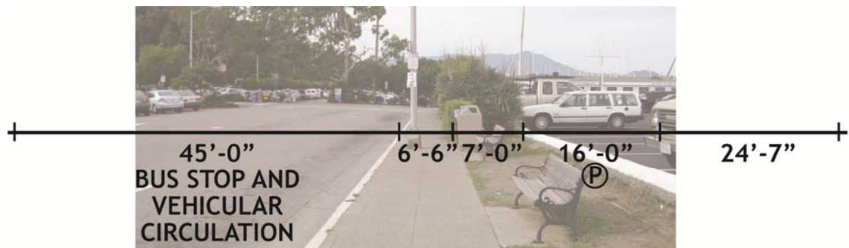
Figure 7-10: Segment 1C Humboldt Avenue - Anchor Street to Bay Street Existing Conditions
