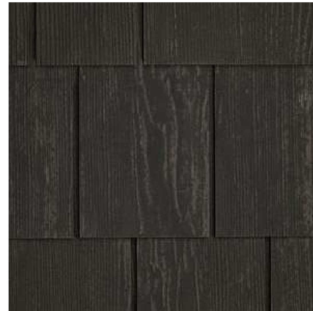
ROOF-01 SHOU SUGI BAN SHINGLE SHOU SUGI BAN IS AN ANCIENT JAPANESE TECHNIQUE THAT PRESERVES WOOD BY CHARRING IT WITH FIRE. AFTER THE WOOD IS CHARRED, IT IS COOLED, CLEANED, AND FINISHED WITH NATURAL OIL.
