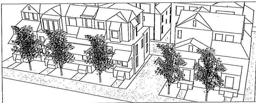
Utilize landscape areas and features to promote energy efficiency. In this example deciduous landscaping provides summer shading.
